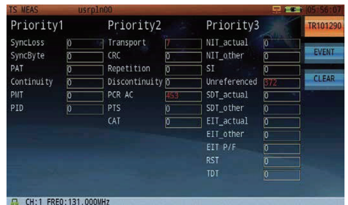
Figure 16: The DS2831 supports transport stream analysis, showing bandwidth usage, basic TS structure, TR 101 290, PiD view, PCR, PSIP, PAT, and PMT tables.
