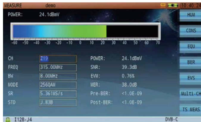
Figure 7: Use DVB-C channel measurements to characterize digital carrier metrics such as channel power, MER, and Pre/Post BER.
