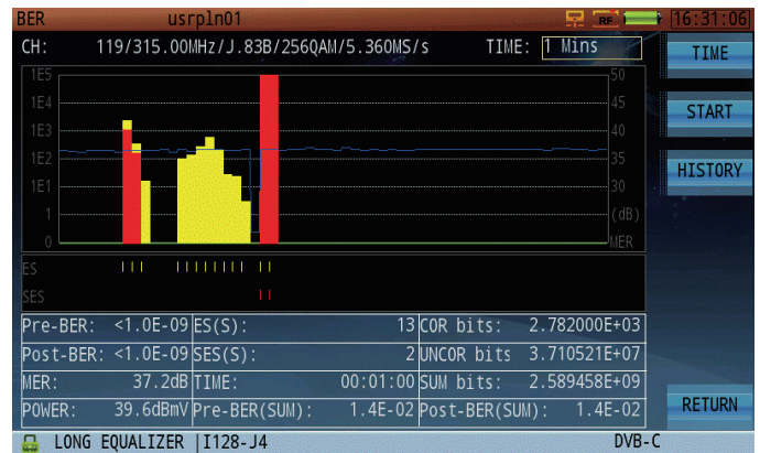
Figure 10: BER and MER Statistical Analysis helps to find impairments, interference and distortions over time.
